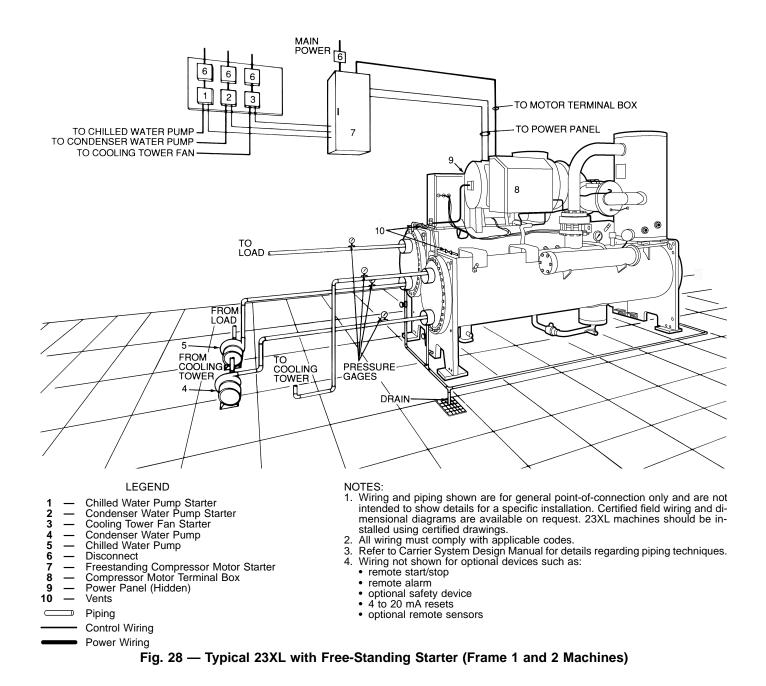
IMPORTANT: Do not insulate terminals until wiring arrangement has been checked and approved by Carrier start-up personnel. Also, make sure correct phasing is followed for proper motor rotation.
